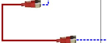
Connect a EIA/TIA 568B between AFF RJ45 socket (GPO1/GPO2), and socket C on SNA50-2 or SNA70. This wiring handles power supply and measuring audio, and switches AFF to SNA mode.
